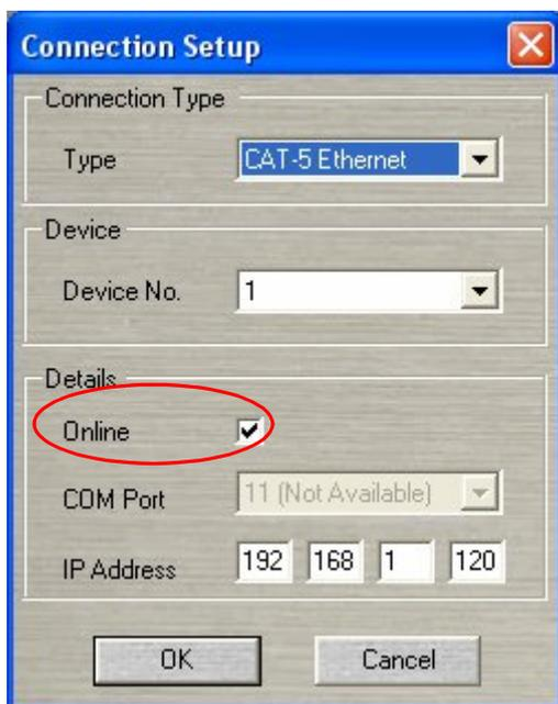
For Ethernet connection, select the following parameters:
